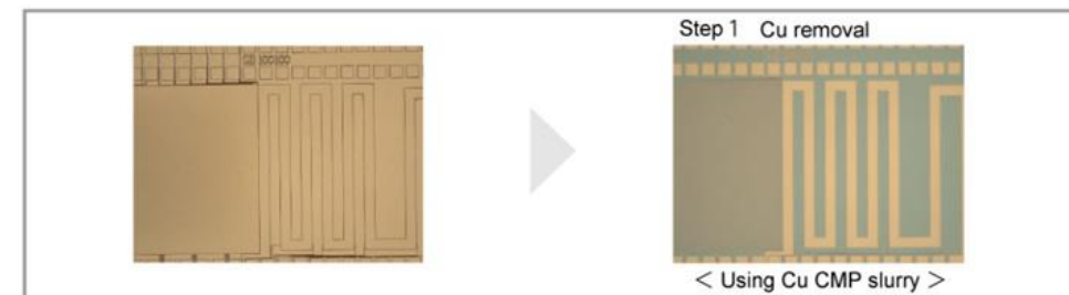
Polishing is stopped on Ta.
